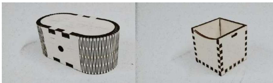
Figure 4. Bending wood and snap-fit patterns.
